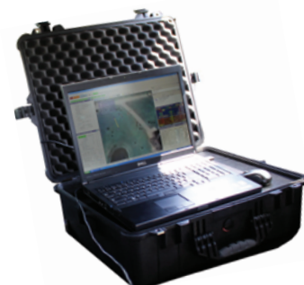
Ground Control Station with Piccolo Command Center
