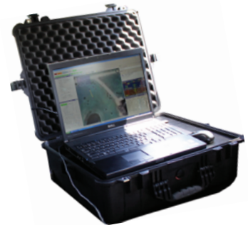
Ground Control Station with Piccolo Command Center
