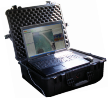
Ground Control Station with Piccolo Command Center
