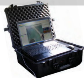
Ground Control Station with Piccolo Command Center
