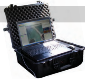
Ground Control Station with Piccolo Command Center
