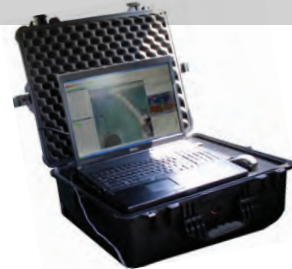
Ground Control Station with Piccolo Command Center
