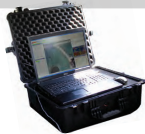
Ground Control Station with Piccolo Command Center
