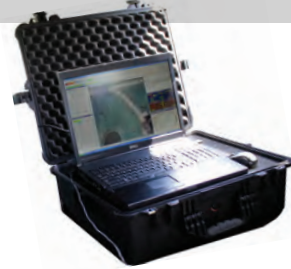
Ground Control Station with Piccolo Command Center
