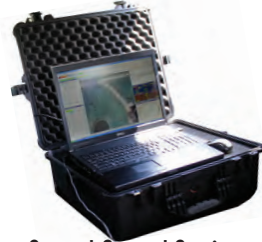
Ground Control Station with Piccolo Command Center
